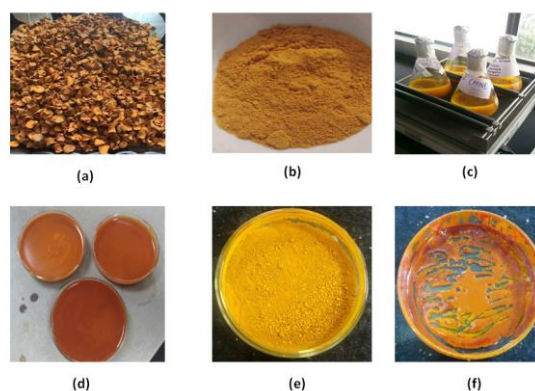
Figure 3: (a) Dried turmeric, (b) Powdered turmeric, (c) Curcumin and acetone loaded on digital shaker, (d) Curcumin obtained after evaporation in rotary evaporator, (e) Solid phase of extracted sample, (f) Semi-solid phase of extracted sample.
